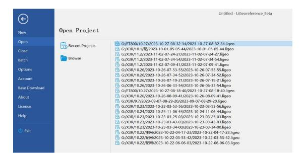
3. After opening the project, the georeferencing tool will automatic import the IMU file.
