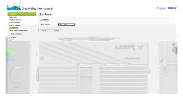
Note: The flight altitude of the web side is selected specifically in the plain area, if the height difference is large in the mountain, you need to choose a higher flight altitude according to the actual terrain relief.
