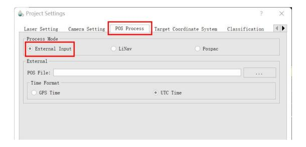
The external input function supports importing the original IMU data and the processed POS data, and the specific format includes \*.pos, \*.out, \*.pof, \*.sbtc, \*.imu. See the figure below.
