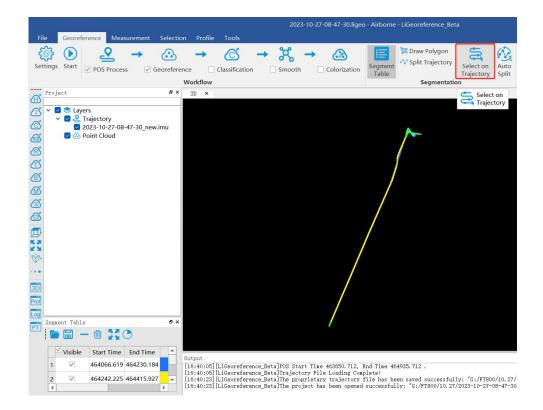
(2) If needed to select multiple trajectories, then repeat the above operation, and the selected trajectory segments will be displayed in the cutting table at the lower left corner.
