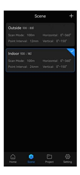
[Scene Name]: Customize the scene name according to different scenarios. [Scan Mode]: The scanning mode can be selected from 100m/280m/600m. [Point Interval]: 3mm/6mm/12mm/24mm can be selected. [Scan Range]: Include Horizontal Range and Vertical Range, Start angle and End angle (in degrees).
