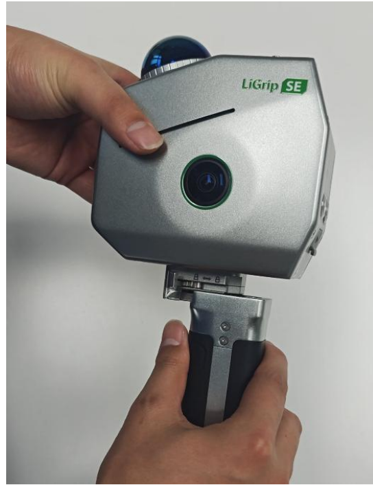
② Align the battery with the slot on the bottom of the device and slide it in.
