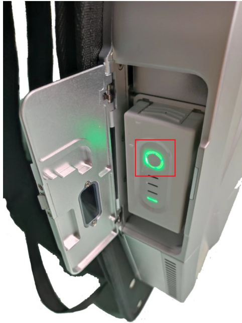
Power on the laser scanner and system
