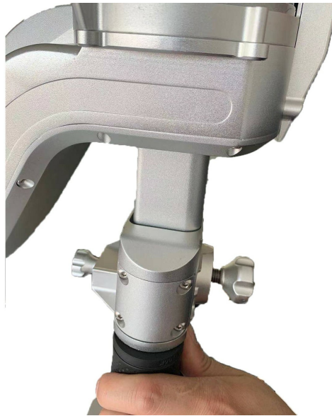
Mount the scanner on main body
