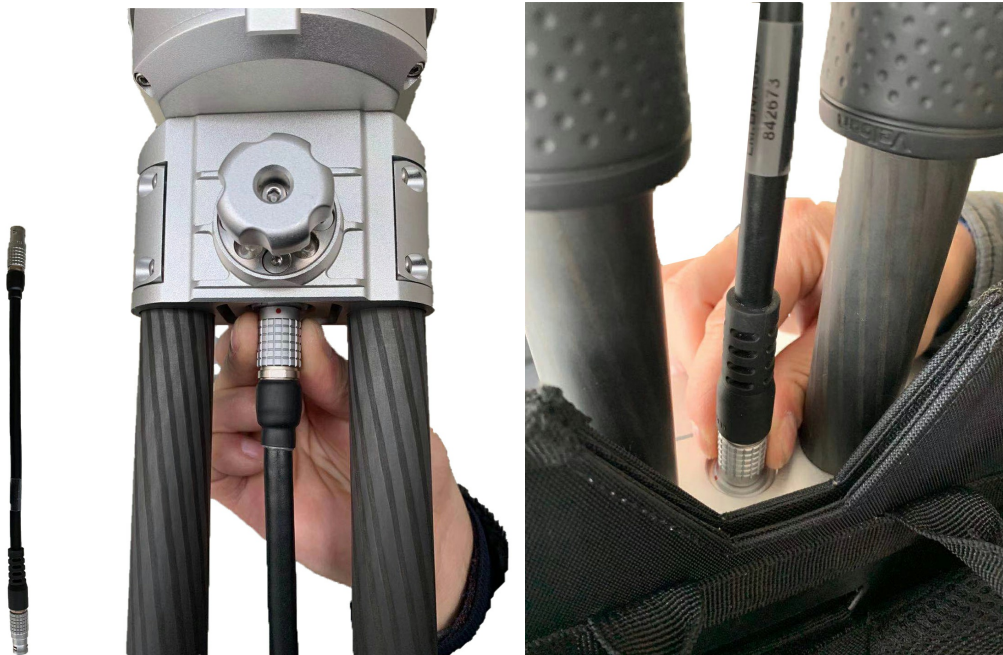
Connect the scanner arm with main body
